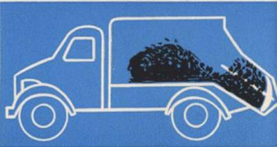
The pusher plate moves the garbage from the hopper into the main space of the truck body and packs it down automatically. The pusher plate is operated hydraulically as soon as the cover and hopper are closed. Having packed the garbage, the pusher plate moves back to the initial position. The pilot lamps located in the cab and on the rear wall of the van body assist the driver in controlling operation of the pusher plate and filling of the body, and ensure safety for the servicing personnel.
