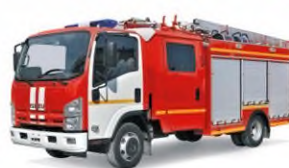
АЦ 1,5-40/2 (ISUZU NQR90L) АС 1,5-40 /2 (ISUZU NQR90L) with the Compressed Air Foam System
