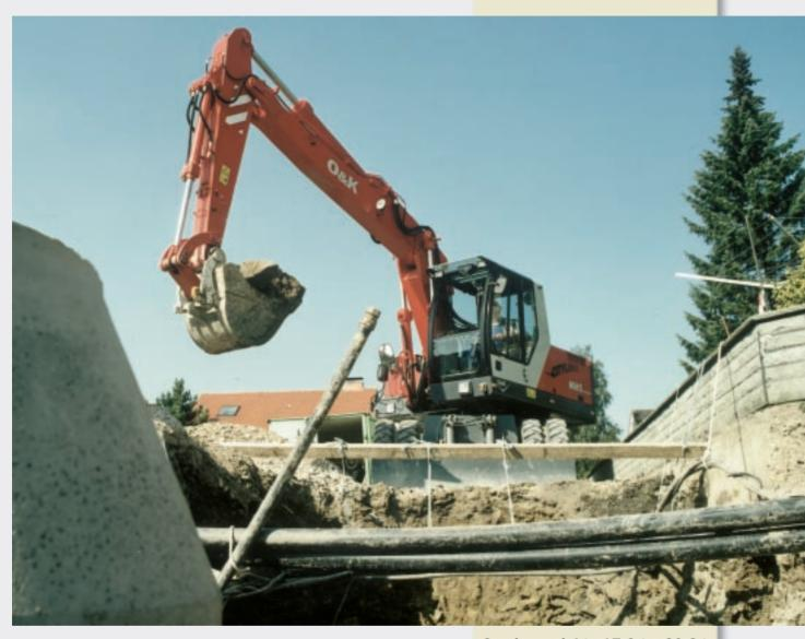
Service weight 17,6 t - 20,8 t Engine output 90 kW Bucket capacities 0,28 - 1,05 m<sup>3</sup> (SAE)
