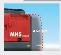
The tail radius is 500 mm shorter when compared with the standard unit. This offers significant advantages, e.g. in road construction, where the second lane must continue to carry traffic. Or for excavation work with cramped space between the buildings. Despite the very compact design, the MH 5 has enormous muscle - a heavyweight in its class.
