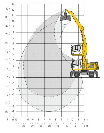
The operating weight includes the basic machine with 4 point outriggers, hydr. cab elevation, 8 solid tyres plus intermediate rings, angled boom 6.00 m, flat angled stick 5.00 m and grab model GM 10B/1.00 m<sup>3</sup> shells for loose material.
