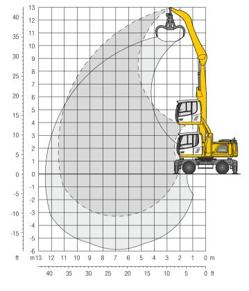
The operating weight includes the basic machine with 4 point outriggers, hydr. cab elevation, 8 solid tyres plus intermediate rings, straight boom 6.60 m, angled stick 5.00 m and grab model GM 65/0.60 m<sup>3</sup> semi-closed tines.
