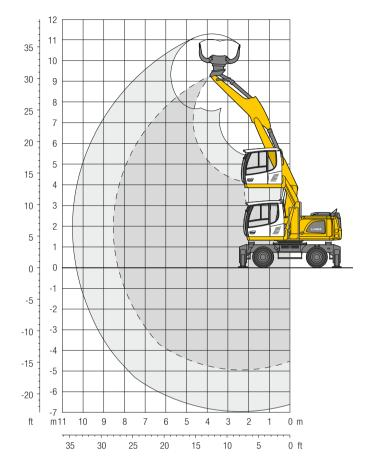
The operating weight includes the basic machine with 4 point outriggers, hydr. cab elevation, 8 solid tyres plus intermediate rings, two-piece boom 3.80 m, stick with tipping kinematics 3.05 m and sorting grab SG 25B/0.55 m<sup>3</sup> perforated shells.
