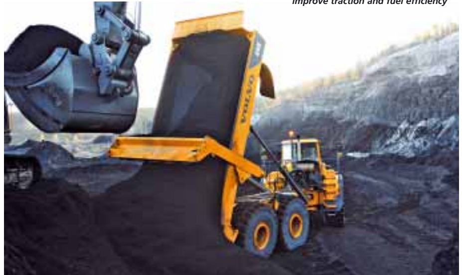
Volvo's A40E has a speed drop box with longitudinal differential and 100% lockup to reduce power losses and improve traction and fuel efficiency
