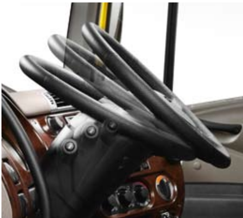
The steering wheel is generously adjustable: 8.5 cm in reach and between 30° and 45° in angle.
