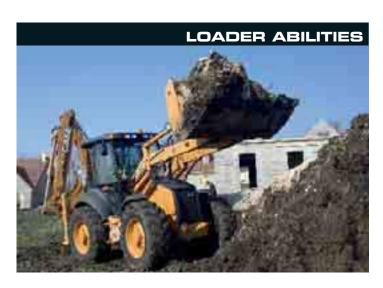
The 695 Super R Series 3 is equipped with a 1,2 m³ loader bucket, which is 20 per cent larger than that on the 580 Super R Series 3 and 590 Super R Series 3 machines.
