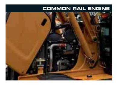
The 695 Super R Series 3 is now powered by the turbocharged Case four cylinder family III engine. This Tier III compliant, climate friendly, high pressure common rail, injected, engine offers a big boost in torque, to 516 Nm, essential for high and tractive effort in tough site conditions. The engine is compatible with the Case Electronic Service Tool (EST), making fault diagnosis a simple task and reducing downtime.
