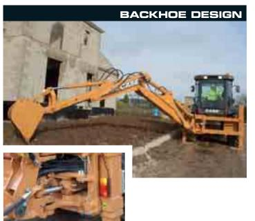
The Super R Series 3 machines have a wide stabiliser frame, offering excellent stability when digging and loading. For maximum rigidity and light weight the Case backhoe uses a robust box type boom design, with all cylinders mounted in line with the boom and dipper to spread effort and prolong component life.
