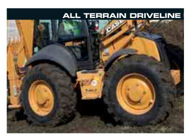
Equal sized wheels create a higher ground clearance across the entire machine. The 695 Super R Series 3 also comes with three mode steering, which allows front steer, all wheel steer, for maximum manoeuvrability, and crab steer which is particularly useful when backfilling and grading.
