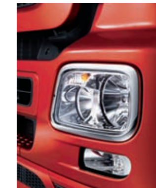
The new Actros' headlamps provide a significantly improved performance, both in range and spread. Full beam performance is particularly impressive, as is the automatic dip beam function that's ideal for quickly changing lighting situations such as driving through tunnels. And for the first time on a truck, Bi-Xenon lamps are also optionally available
