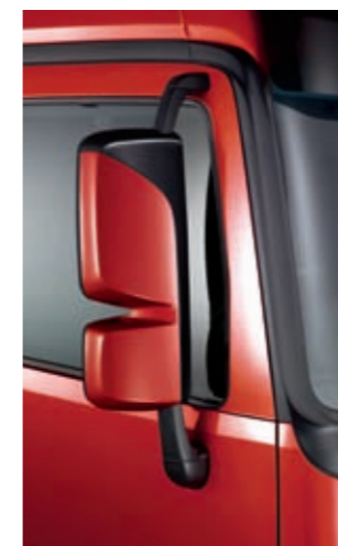
Improved exterior mirrors give a better than ever view down the sides of the vehicle. The standard finish for the covers is in black, with the option of painting into the chosen cab colour. Mirror assemblies for Executive specification trucks have a chrome finish
