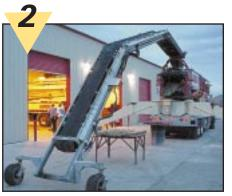
Raise the feeder hinges as high as possible, or until the stack valve is nearly out of reach. This will allow enough slack in the belt to release the belt tension.
