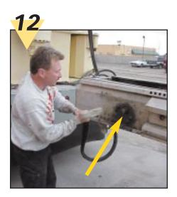
Refer to the Telebelt Manual Maintenance Section 6.11 for the complete procedure for removing and installing the feeder collet.
