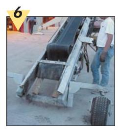
Slowly retract the dolly. This will push the tail pulley frame into the side rails. Do not push the frame so contact is made with the first u-roller. When the frame is positioned as shown, there is plenty of room to remove the tail pulley.
