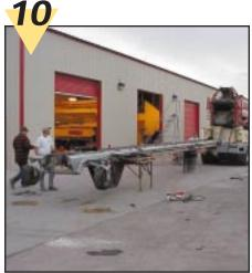
Lower the feeder to suitable work stands (horses) in order to remove the pulley and feeder belt. Operating the hinges and dolly can make setting the feeder in place much easier. When the feeder hinges are straight, shut off the truck engine and remove the keys.
