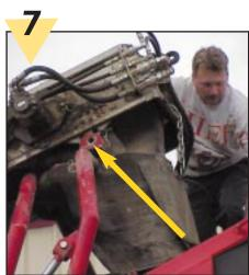
Attach a suitable lifting device to the top section of the feeder.
