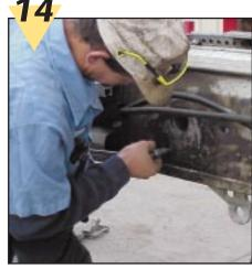
Keep clear of the underside of the belt in case the pulley drops out when the bolts are removed.
