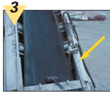
Tap the tail pulley slide frame to loosen the bolts. It might be necessary to use a tensioning jack to move the slide enough to loosen the bolts.
