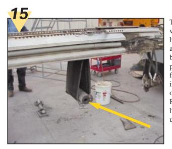
The pulley assembly will drop down and be held by the loop at the end of the belt. Remove the pulley assembly from the loop and inspect for bearing or nilos ring damage. Replace damaged bearings and seals upon reassembly.
