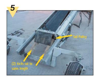
Straighten the feeder hinges. Cut two 4 x 4 boards to equal lengths (about 18" to 24").
