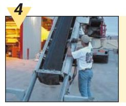
Remove the hair pins from one side of the three hopper u-rollers.
