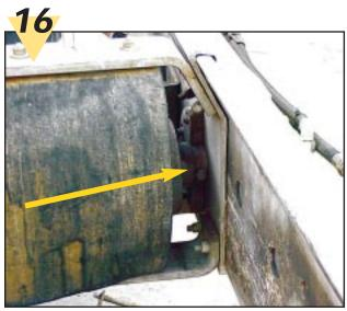
Stay clear of the underside of the belt for this step. Depending on the year of manufacture, there will be either a 5/16" or M16 bolt at each end of the tail pulley. Remove the bolts and the tail pulley. Once the tail pulley has been removed, the old belt can be removed and rolled up.
