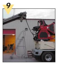
Keep the feeder hoses away from projections and pull the truck ahead enough for clearance. Set the parking brake and re-engage the right-hand PTO.
