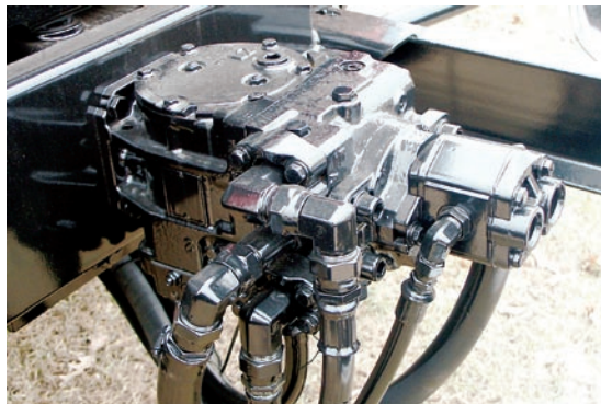
Optional 4.57 CID (90 Series) with 2.1 CIU motor
