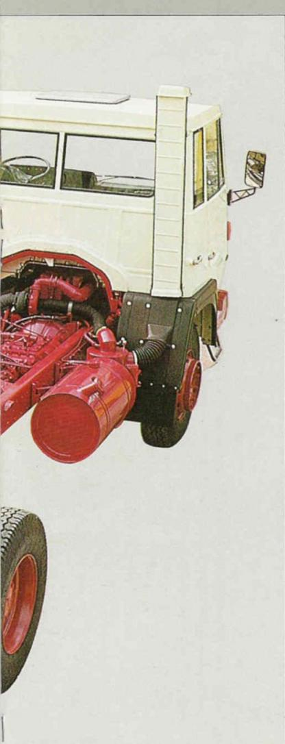
This comfortable road behaviou is also enhanced, moreover, by the steering geometry and the small unsprung masses of the chassis units as well as by the self-centering feature of the wheel hub and the consequent absolutely true running of the wheels. 15-degree taper-base rims result in a weight saving of up to 30 kg per wheel. All chassis units of the Steyr Puch Trucks of the Model Series 91 are equipped with braking systems that conform to EC-directives: hydraulic dual-circuit brake with dual-
