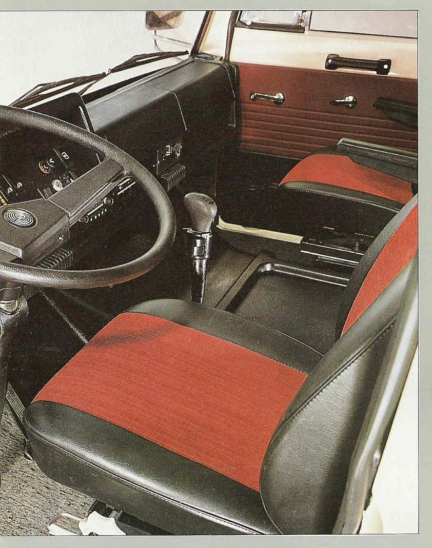
\* the manual force required in order to move the steering wheel amounts to only 8 kp \* the steering wheel rim has been amply covered with foamed plastic \* the bunks in the long-distance driver's cab are not only of anatomically correct shape but also padded and upholstered with material that is permeable to air and thus able to "breathe" \* fitted with sun visors or roller blinds as preferred.
