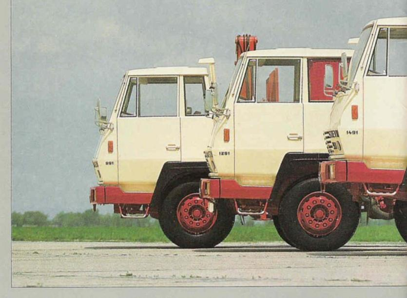
In evolving the design concept of the Model Series 91, the well-tried Plus-driver's cab, which is absolutely tops as regards its comfort and safety features, has been retained. Whatever additional refinements were feasible in regard to the shape and design of this cab have been implemented: all driver's cabs of this model series have been made tiltable by 70 degrees; they can be tilted with ease and locked in place securely (triple security) regardless of the gradient or tilt of the vehicle.
