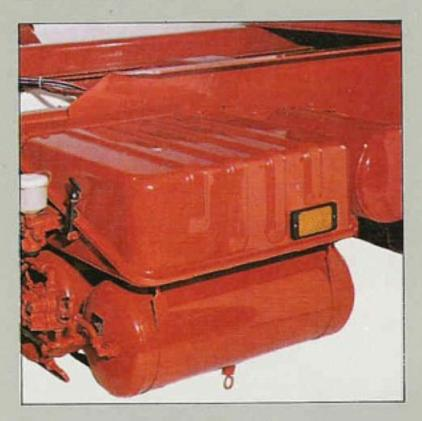
grouping of such assemblies as braking system, battery case and exhaust so as to form a single modular unit. The chassis units are available in variants of all types and descriptions, i.e. as 2- or 3-axle models in normal and all-wheel-drive versions, with various wheelbases, design variations and wheel combinations 4x2, 4x4, 6x2, 6x4 and 6x6. The elastic parallel-ladder-type frame, which is of double strength throughout the supporting sections, features top chords that are
