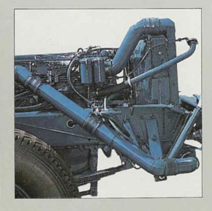
The Steyr-central-turbulence combustion process and the charge-air pressure-dependent fuel quantity injected are only two of several measures contributing to improved combustion efficiency and leading to an optimal specific fuel consumption of 204 g/kWh (150 g/hph) with charge cooling.
