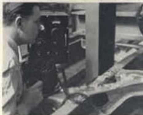
Every new type of frame is subjected to meticulous tests and investigations. Stress measurements make the strength properties of the frame an open book to the engineering staff of Boeing-Lab.
