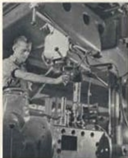
All holes in the sides of the transmission are drilled in a radial drilling machine.
