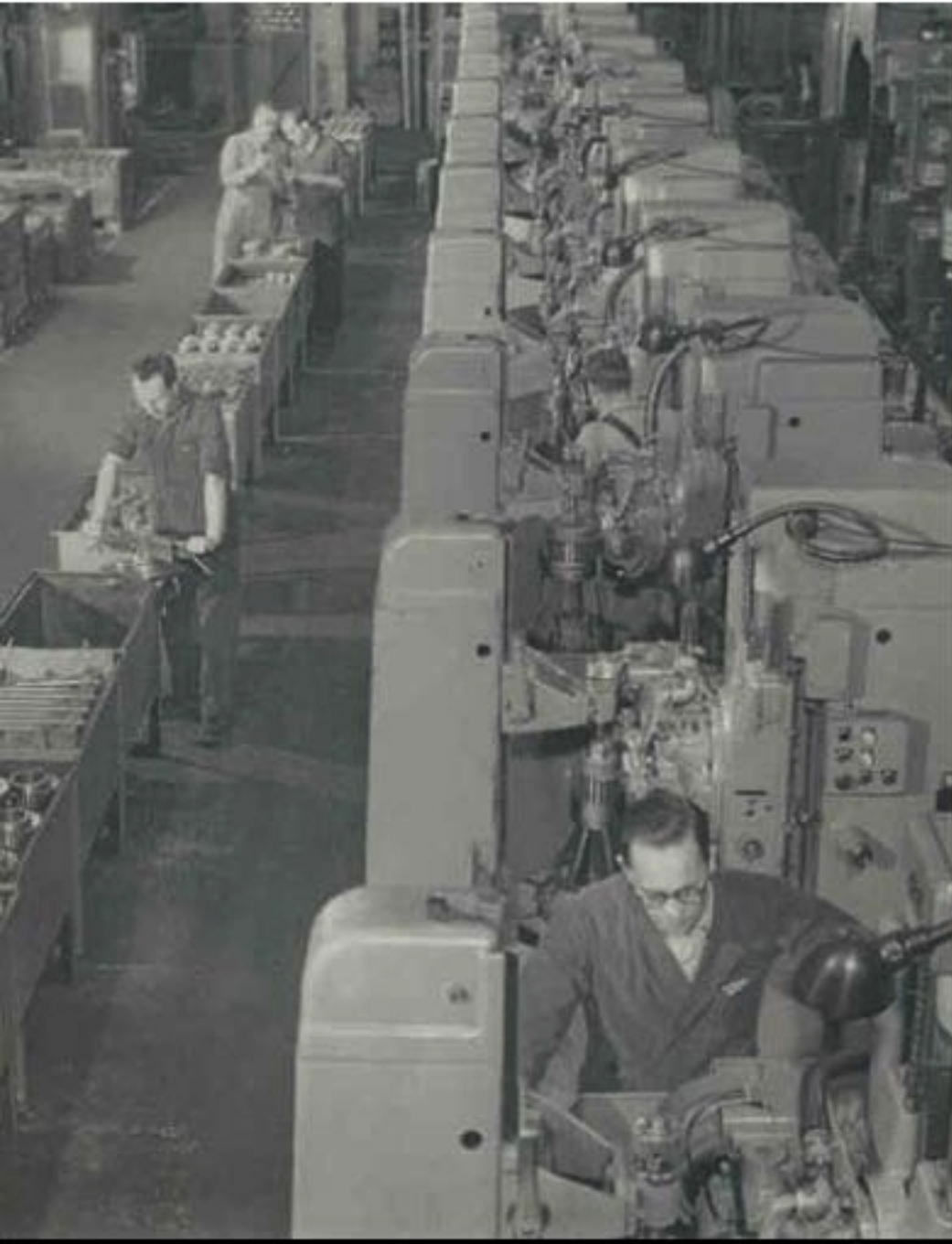
Precision machines cut the teeth on the turned gear and shaft blanks.
