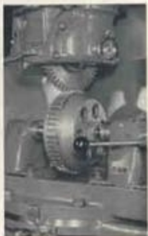
Special machines grind tiny small grooves in the slope of the tooth and give them their final surface finish.
