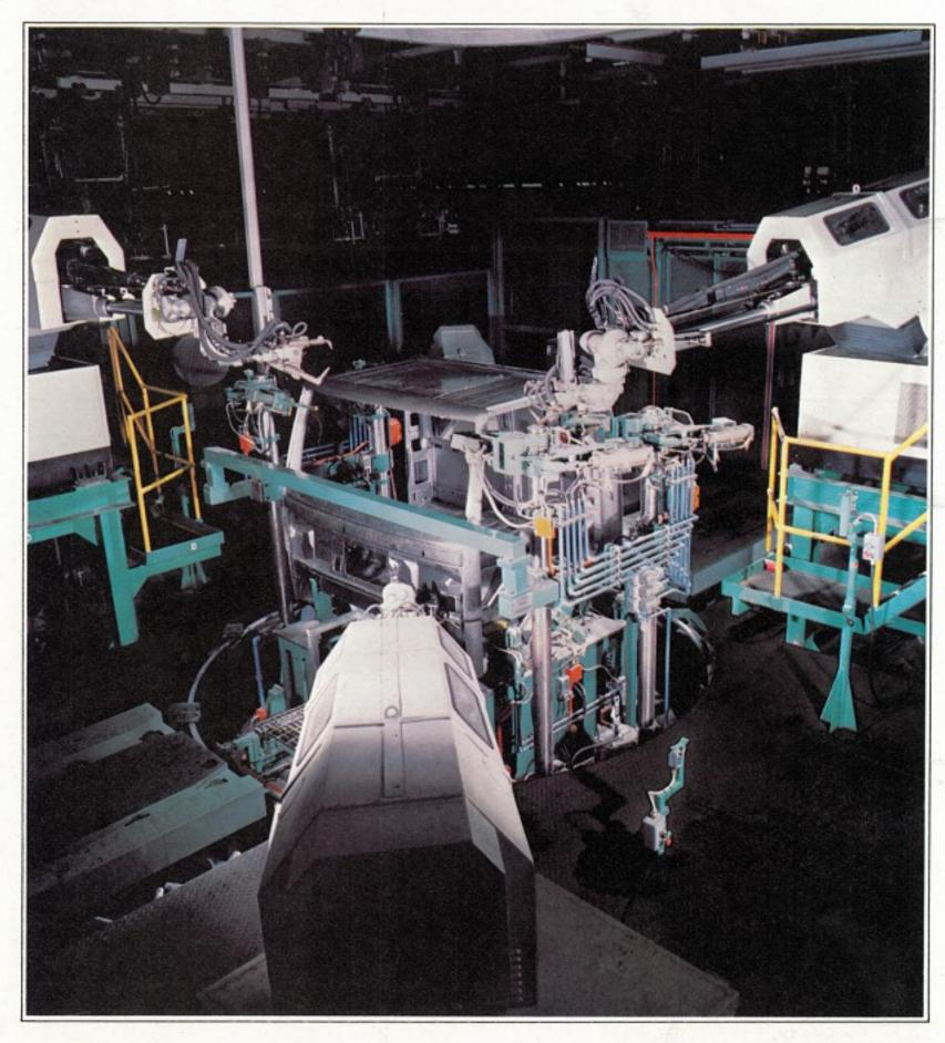
Electro painting is carried out using a cathodic process and this is the key factor in the success of our anti corrosion treatment. Cathodic primers are themselves chemically superior as rust inhibitors than the anodic primers used are then sealed with a PVC in most other processes.
