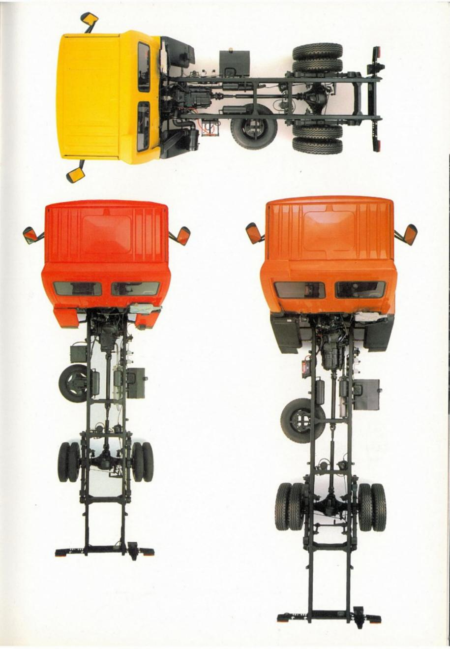
Just as protrusions above the frame have been eliminated so has equipment outside the frame been minimised.
