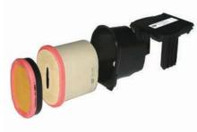
**Air Cleaner.** A new, dry-type, axial seal air cleaner with automatic, integrated dust ejection system provides more efficient pre-separation. The two-stage air filter incorporates both air cleaner and precleaner functions into a single unit mounted under the hood.
