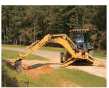
Backhoe Boom. The excavator-style boom features box section fabrication with internal stiffeners for better balance and weight distribution. The curved design provides additional clearance over obstacles while digging a trench or truck loading. The narrow boom enhances the viewing area to the bucket and trench throughout the entire operating range.
