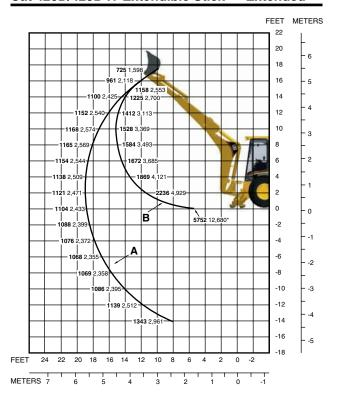
Lift capacities are over-end values. Machine equipped with 2WD, OROPS, 0.96 m³ (1.25 yd³) general-purpose bucket, and 355 kg (780 lb) counterweight. Extendible stick includes 567 kg (1,250 lb) counterweight.
