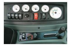
**Operator Controls.** The controls of the 420D/420D IT have been carefully laid out to create a user-friendly environment. Switches, boom lock and pilot operated stabilizer controls are located in the side console, within easy reach of the operator. White-faced gauges are easy to read and the low effort pilot controls reduce operator fatigue and help boost overall productivity.
