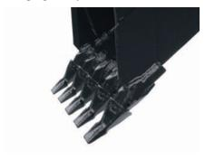
New DRS 230 (Diagonal Retention System). New DRS 230 with wide adapters provides maximum strength and improved wear characteristics. Heavy-duty bucket teeth are attached with diagonal pins rather than horizontal pins for easy exchange. The adapters are stronger as a result of this improved diagonal pinning and additional wear material on the bucket teeth increases durability.
