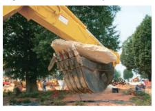
**Bucket Characteristics.** The side profile has a scalloped edge, similar to an excavator bucket, for exceptional fill factor characteristics and secure clamping ability.
