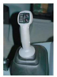
**IT Loader Controls.** The 420D IT has a new, standard single lever, pilot-operated loader control for proportional control and fine modulation of the hydraulic work tools. A thumb roller control on top operates auxiliary hydraulic functions such as the clam bucket and two buttons control hydraulic broom angle.
