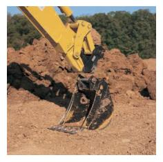
Quick Couplers. Allow for quick attachment of buckets and other work tools. The D-Series High Rotation pin grabber design and a C-Series compatible pin grabber allow buckets to be changed without removing the bucket pins. Other manufacturers' buckets can be coupled with a pin puller coupler, one for Case and D-Series buckets or one for John Deere and D-Series buckets. D-Series quick couplers are painted black for easy identification.
