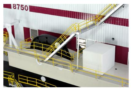
The 8750 scale model features a fully detailed eccentric-cam walking system, with the walking shoes in a raised "fixed" working position, allowing full rotation of the upper works on the machine base, better known as the "tub."
