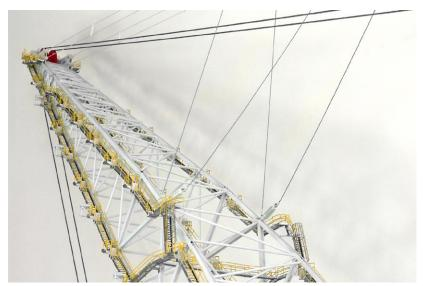
The 8750 dragline features fully detailed walkways running up and down each side of the main boom. No attention to detail has been overlooked in the design of the "4-chord" boom structure itself, which is both strong and lightweight in construction.
