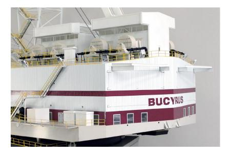
This rear view of the 8750 highlights the metal louvered vents that run across the lower portion of the housing, just above the revolving frame structure.
