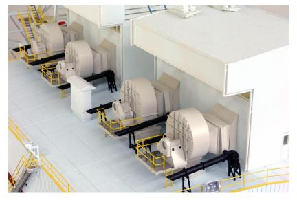
The roof top is equipped with exposed air filter assemblies which are used on the real dragline for pulling in air through the filtered intakes into the pressurized housing. There are eight air filtration fan assemblies; four per side, each with two scavenge fans, all with fully detailed photo-etched catwalks with metal railings.
