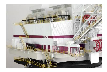
The 8750 is equipped with a fully detailed extended operator's cab mounted on the right side of the upper frame structure.
