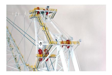
The main hoist ropes run on sheaves mounted on the tri-structure boom support, and are manually operated by inserting a key into the left side of the housing. The main drag ropes are also operated in this same way. The robust tri-structure boom support holds up the weight of the main boom by means of four heavy-duty boom-point lines.
