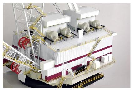
The housing of the model features all of the major detail found on the real Bucyrus 8750, such as the operator's cab, electrical cabinets, walkways, and fully detailed rooftop air filtration system.
