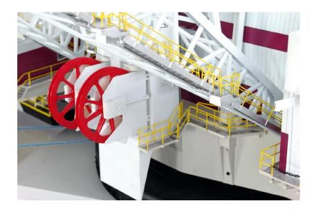
The large front-mounted lower sheaves of the overand-under fairlead structure are pinned in place on the revolving frame so they can swing from left to right to match the pull of the drag-ropes.
