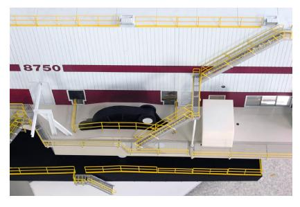
The upper portion of the eccentric cam of the walking system protrudes through the revolving frame deck and is clearly visible from either side of the model. Each cam has a walking shoe attached to it, featuring details such as railings and steps.
