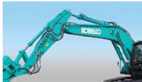
High-strength multi-dismantling attachment
