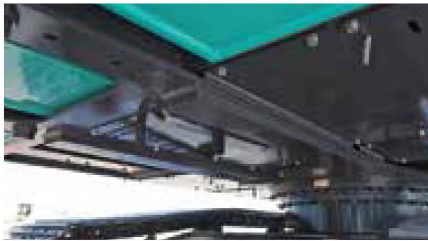
Frame is reinforced from the factory to support the heavier counterweight.
