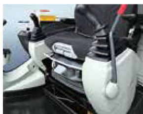
Suspension seat absorbs vibration
