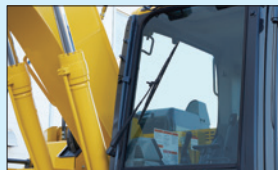
Remote intermittent wiper with windshield washer
