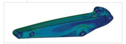
Booms and Arms have been redesigned using advanced CAD (Computer Aided Design) and FEM (Finite Elements Methodology) Systems to get higher strength **only** in those areas where stress is concentrated.
