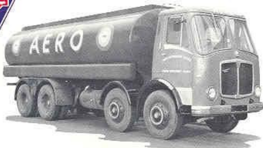
Aero Motor Spirit's A.E.C. "Mammoth Major" 6-wheel tanker. Another example of the Mark V, with its driver entrance ahead of the front axle, deep curved windcreens, and other design features contributing to increased reliability and driver comfort. Its tank capacity is 4,000 gallons.
