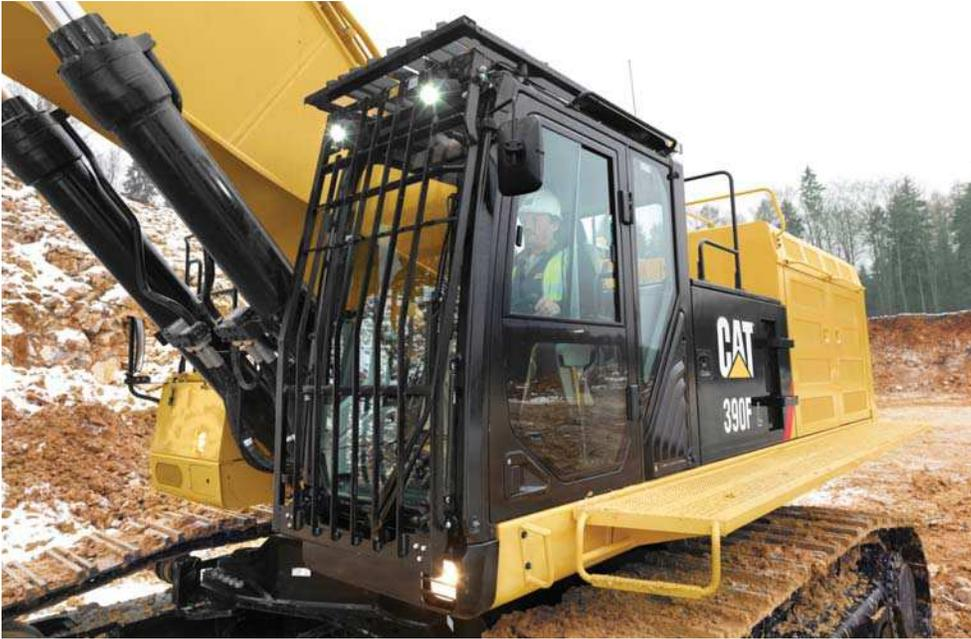
Optional Falling Object Guards (FOGS) further protect you from debris coming to the cab.
