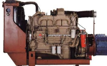
The engines are easy to reach, service and remove, they rest on two independant cradles.
