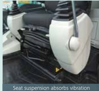
Seat suspension absorbs vibration
