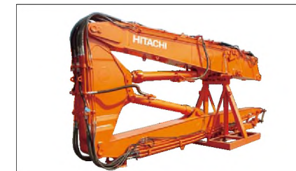
High reach demolition stand
