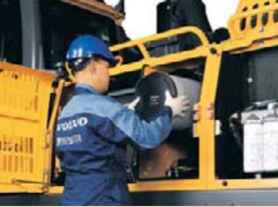
• Simplified, ground level service access.
