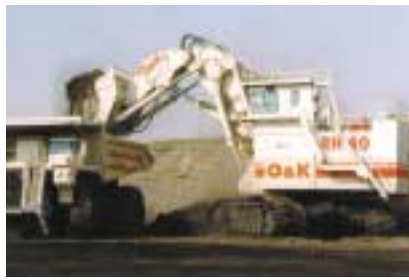
RH 400-5: the first machine with electric drive in a coal mine, USA
