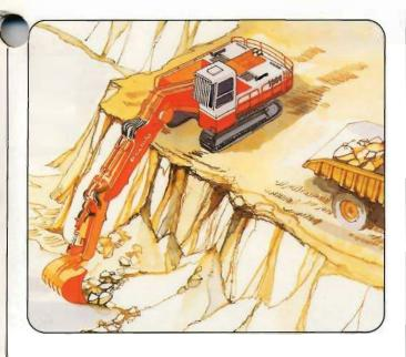
3. The Poclain 1000 with backhoe attachment on top of the bench with the truck at the same level. This application allows you to keep the job going when the weather conditions would normally prevent the trucks circulating on the lower level, due to water or mud. Even though the cycle time being longer, you keep your production going.
