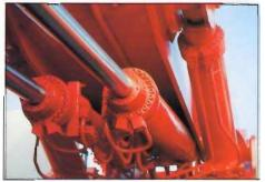
all grease points on the upperstructure and attachments. Replacement of the grease drum is easy to handle with the Poclain 1000 winch. This central lube system will not forget a greasing point.
