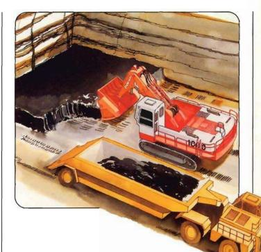
4. In sedimentary mines, such as coal, you can follow very precisely the seam of coal. The high penetration force of the 1000 allows you to dig without blasting or ripping, you avoid pulverizing the coal, which means less fines and higher production of finished product.
