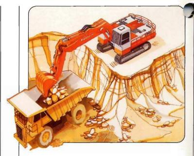
2. The Poclain 1000 with backhoe attachment, dumpers positioned at the lower level. The best position to extract materials difficult to work at the foot of the face. It's the position which allows the most selective digging. The narrow bucket gives you the best penetration force and the shortest cycle time resulting in a production equal or even higher than the shovel attachment.
