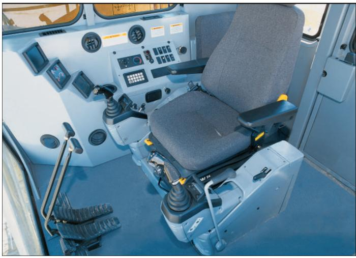
Spacious operator compartment measures 1790 mm (5'10") wide by 2178 mm (7'2") long by 2236 mm (7'4") high and has an exceptional, unobstructed view of the bucket and loading area.
