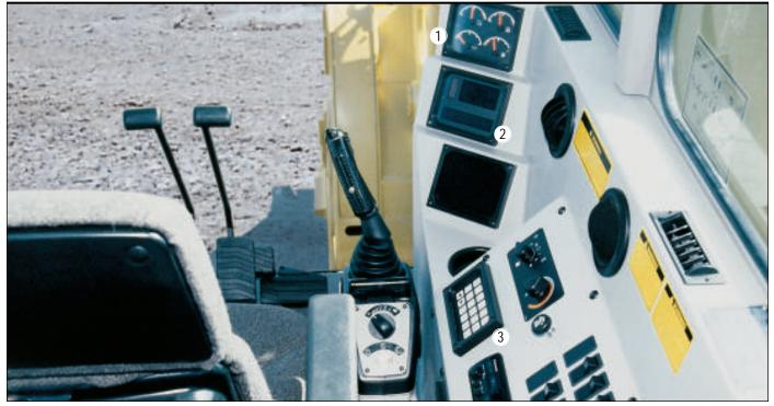
The VIMS system continuously displays critical machine data. This information can be used to keep the 5130B performing at top production levels.
