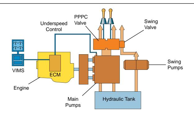
Exclusive Caterpillar Proportional Priority Pressure Compensating (PPPC) valves are used in both the front structure and travel systems.
