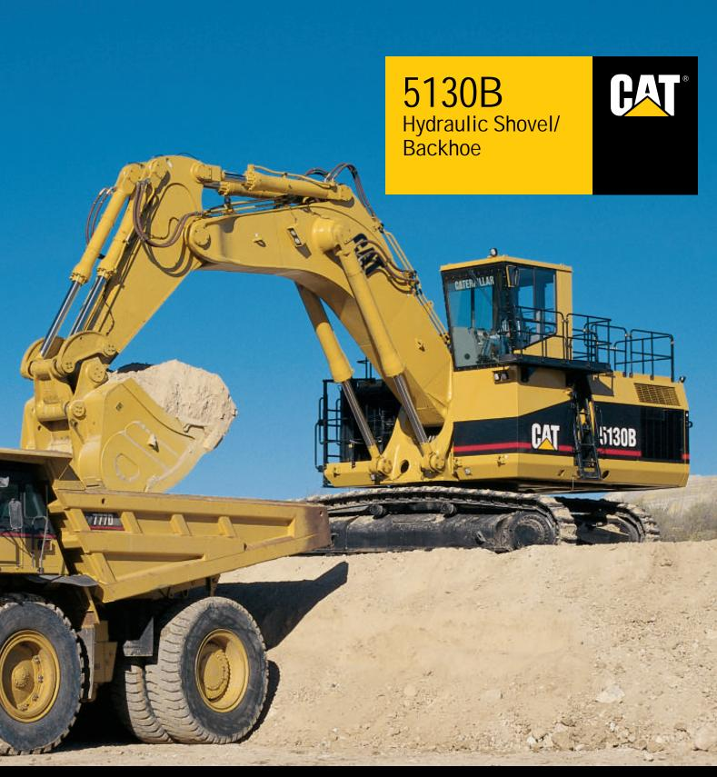
Available in Front Shovel and Backhoe configuration, the new Caterpillar® 5130B is primarily matched to the Cat® 777D truck, but can also be teamed with the 773D or 775D and other trucks in the 65 to 100 ton size class. This makes for efficient loading and hauling systems for mining, quarrying and heavy construction applications.
