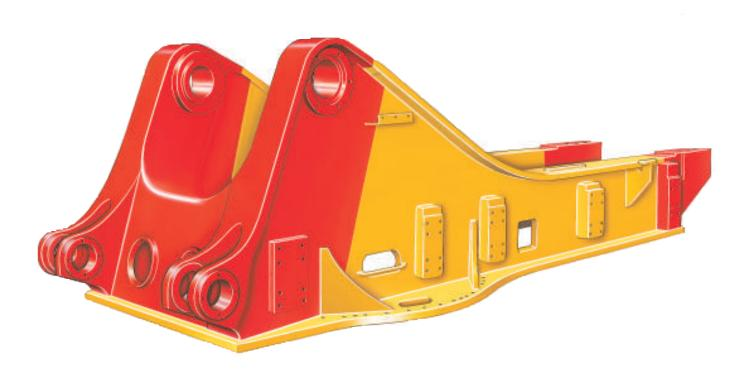
Heavy-duty castings are used extensively in high-stress areas for excellent, long-term structural durability.
