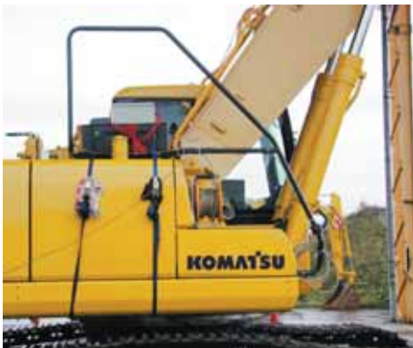
High reach demolition machine, carrying test instrumentation.
