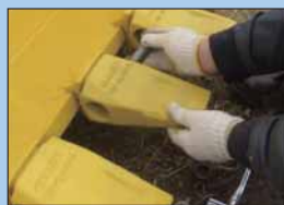
Insert exclusive pin to the adapter pin hole
