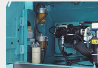
● Firewall separates the pump compartment from the engine
