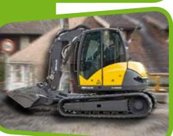
And when transporting you 8MCR, a simple 6X4 or an Ampirol trailer are all you need, you can load your 8MCR and its equipment onto your lorry without difficulty.
