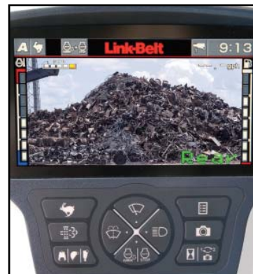
Rear-view camera displays a panoramic view of work area for improved safety
