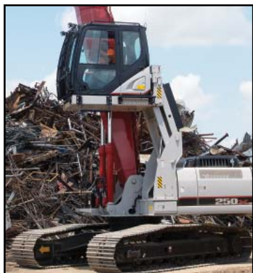
New boom up cushioning valve and shock-less cab riser design improve operator comfort and control
