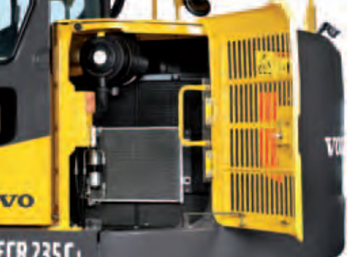
• Ground level air filter access.
