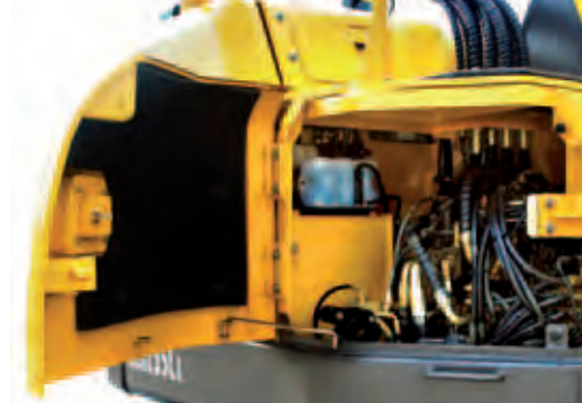
• Wide open, ground level service area provides easy hydraulic valve access.
