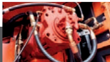
Hydraulic pump The main pump has a capacity of 2 x 436 l/min
