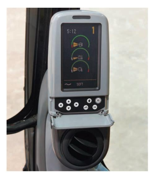
**Monitor Display Screen.** The monitor is a full color 400 x 234 pixels Liquid Crystal Display (LCD) graphic display. The Master Caution action lamp blinks ON and OFF when one of the critical conditions below occurs:
