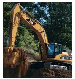
**Tracks.** The 330D comes standard with grease lubricated tracks. The track links are assembled and sealed with grease to decrease internal bushing wear, reduce travel noise and extend service life lowering operating costs.
