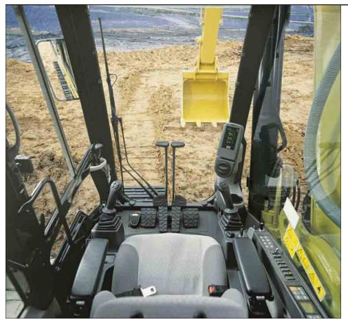
**Operator Station.** The workstation is spacious, quiet and comfortable, assuring high productivity during a long workday. The air conditioner and attachment switches are conveniently located on the right-hand wall, and the key switch and throttle dial are on the right-hand console. The monitor is easy to see and maximizes visibility.
