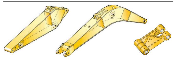
Front Linkage Attachments. Select the right combination of front linkage with your Cat dealer to ensure high productivity from the very start of your job. Three types of booms and six sticks are available, offering a range of configurations suitable for a wide variety of applications and offer a large combination of reach and digging forces for optimum versatility. All booms and sticks undergo a stress relieving process for greater durability.
