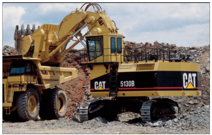
**Shipping and assembly.** Machine breaks down into eight modules for ease of shipping.
