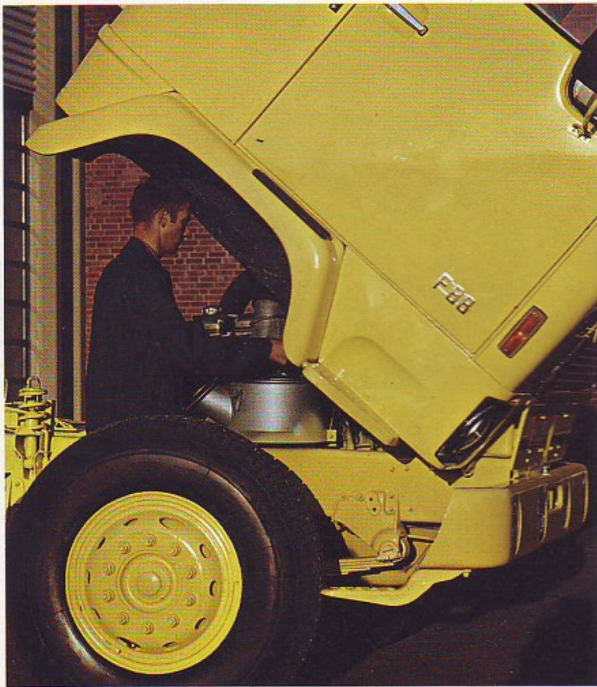
When the cab is tilted out of the way, the engine, gearbox and front end are readily accessible. The robust torsional springs facilitate tilting of the cab. In the case of the sleeper cab, extra equipment available includes a hydraulic tilting device.
