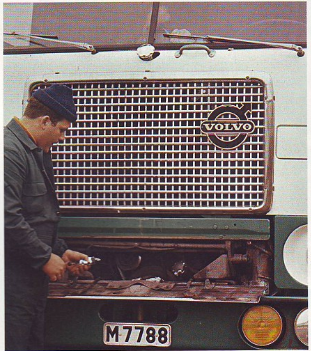
Daily checking can be carried out without it being necessary to tilt the cab. The oil dipstick and oil filler, for example, are readily accessible through a servicing cover in the front of the truck.
