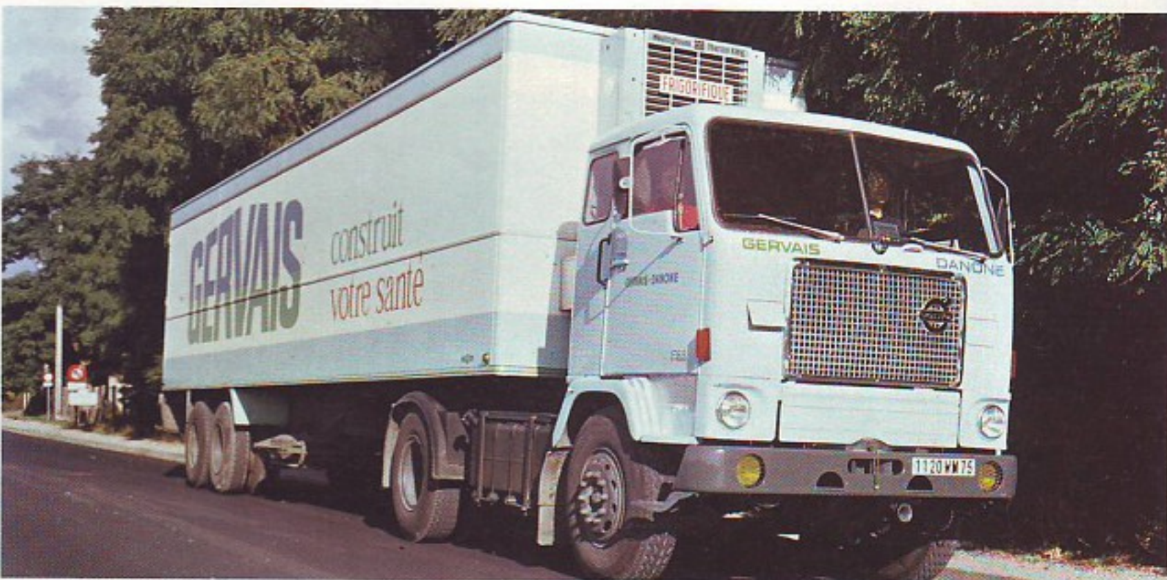
F 88-32 as tractor unit for use with semi-trailer. TD 100 engine, SR 61, double reduction final drive. (France)
