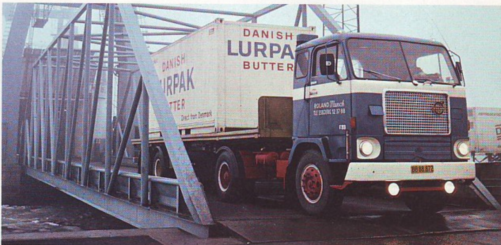
F 88-32 as tractor unit for use with semi-trailer designed for container transport. TD 100 engine, R 60 gearbox, double reduction final drive.
