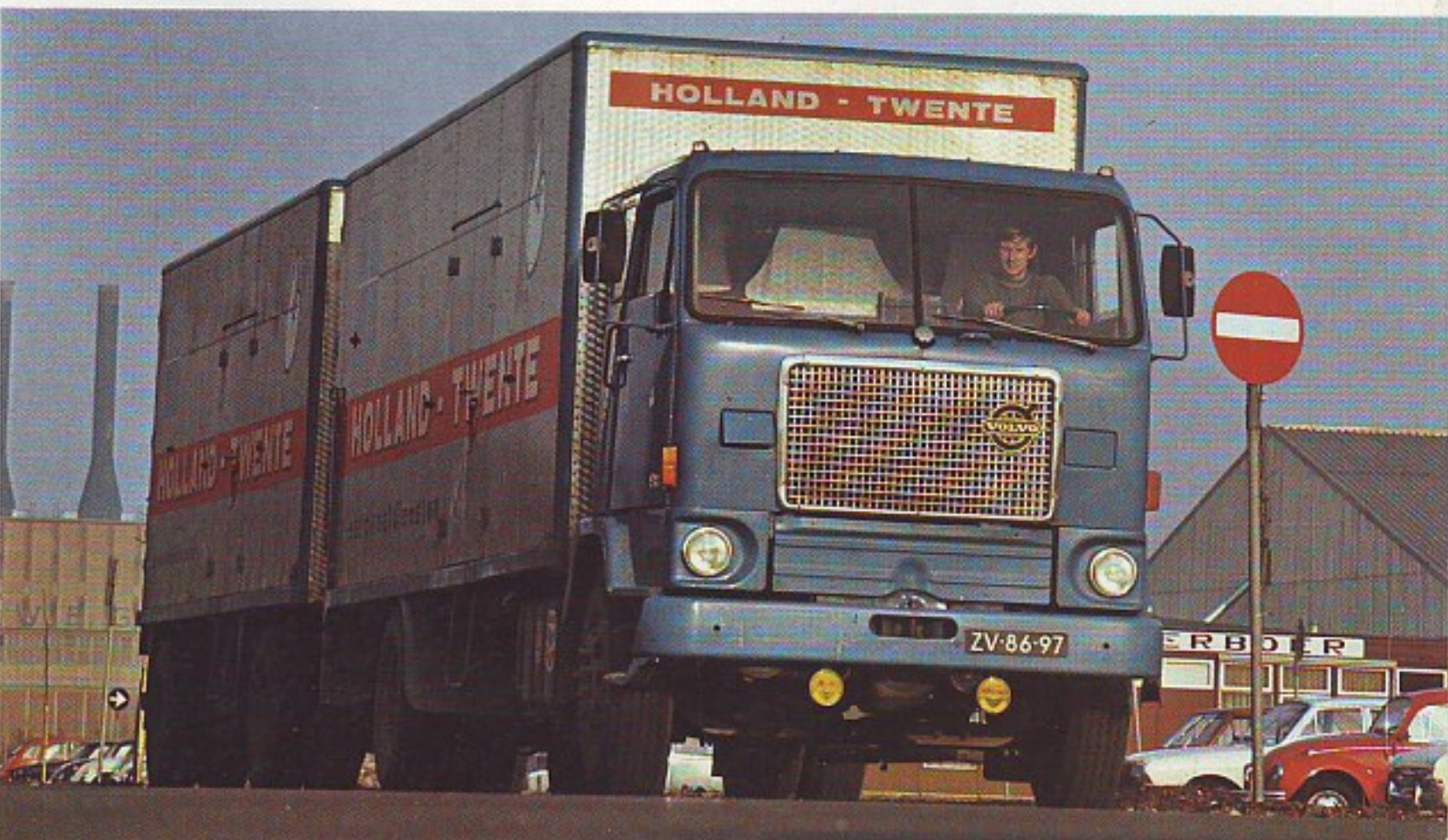
F 88-49 with van body and two-axle trailer. TD 100 engine, SR 61 gearbox, double reduction final drive.
