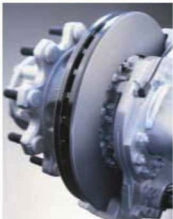
Ventilated disc brakes on the front and rear axle.
