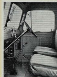
An interior view of the normal control cab for Bedford models K, MS, and ML.
