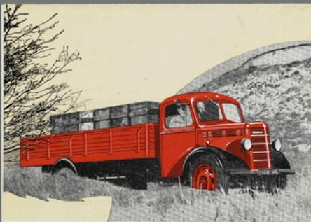
Above—A Bedford model OLEB Dropside Truck which can be converted to a Flat Platform Truck.
