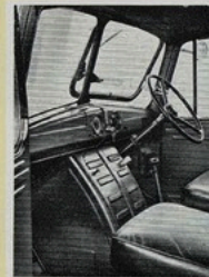
As shown above, driving controls are in the normal position on the semi-forward control cabs on Bedford O models.
