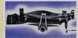
Models OSB and OLB have heavy duty helper springs as illustrated above.
