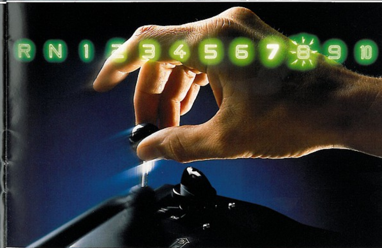
CAG, the Scania Computer-Aided Gear changing system, combines the convenience of the automatic transmission with the fuel-pinching performance of the manual unit.
