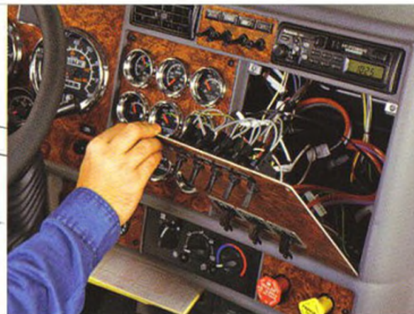
Modular dash panels tilt out to expose cab wiring that is color-coded and numbered for quick circuit tracing. Gauges are front-loading with push-on connections, a cinch to replace.
