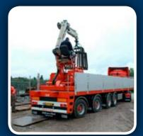
If more load capacity is required, the Floor **C-LINE** crane trailer can be equipped with 4 axles to provide a technical capacity of 54 tonnes. If you want to avoid overloading your tractor, the patented Floor Payload Adjusting System (PAS) is an excellent tool. This system ensures that the fifth-wheel pressure of your tractor is optimized automatically. It is available on all 4-axle **C-LINE** Crane Trailers.
