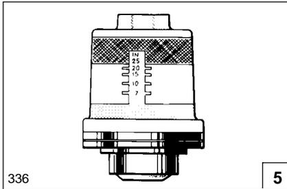
**5. Air Cleaner Restriction Gauge** - Indicates the degree of restriction as the yellow band rises in the gauge window. The filter element should be cleaned or replaced if the yellow band locks in place when the engine is shut down. Reset the gauge by pressing button on gauge with engine running.
