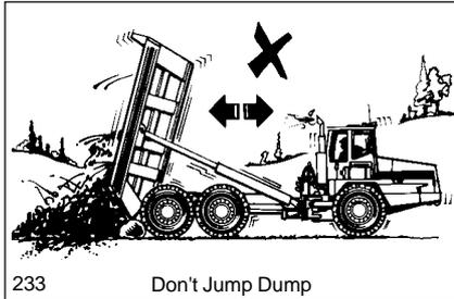
Never 'JUMP DUMP' the machine by bouncing the rear tyres against a stop block, or otherwise jarring the body in its raised position, to dislodge stuck or frozen material. The tremendous loads that this practice develops on the body pin area, chassis and hydraulic system can cause needless, extensive stresses.
