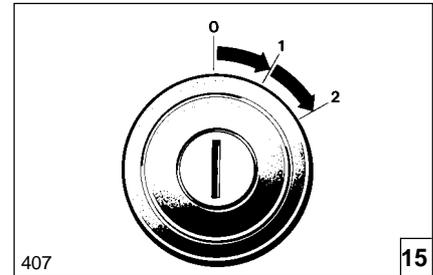
**16. Battery Master Switch** - (Located on the left hand side of the tractor frame) Turn key clockwise to connect the batteries to the electrical circuits. Switch key off and remove when leaving vehicle unattended.
