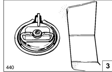
**3. Radiator Top Tank** - Check Coolant Level.
