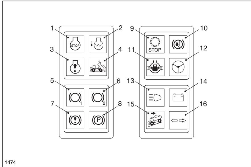
**6. Trailer Brakes Overstroke (Red)** - Illuminates if the brake system pressure is low. A buzzer also sounds. If light illuminates, stop vehicle and investigate the cause.
