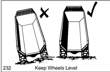
Before raising the body, make sure that the rear wheels are on firm level ground. If one wheel is higher than the other, a twisting strain is imposed upon the body hinge pins, hoists and chassis. Stop the machine, allow the engine to slow to idle, shift the transmission to 'NEUTRAL' and apply the brakes with the Parking-Emergency Brake control, to hold the machine stationary.
