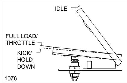
When shifting from 'NEUTRAL' to start from a standstill, or to reverse direction, decelerate the engine to idle speed before selecting the proper gear. When 'REVERSE' is selected, the 'Reverse Alarm' sounds and the 'Reverse Light' illuminates to warn personnel to the rear of the machine that reverse gear has been selected.
