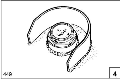
**4. Fuel Level Gauge** - Indicates the level in the fuel tank. Capacity 463 litres (122 US gal). Fill the tank before parking the vehicle overnight to minimize condensation in the tank. Avoid a dry tank condition which requires bleeding the fuel system.
