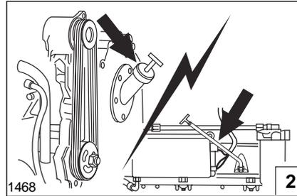
**2. Engine** - With engine off, check engine oil level. The oil level should be up to the upper dot on the dipstick. If the level only reaches the lower dot, the oil should be topped up immediately.
