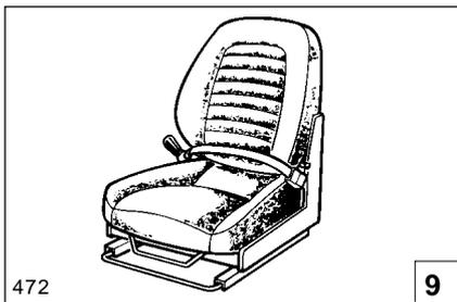
**9. Seat and Seat Belts** - Adjust the seat position and lap belt, as required, to allow complete machine control at all times with minimum fatigue. Make sure the seat belt does not restrict movement for proper machine operation.
