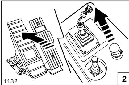
1. Make sure the body is fully down and the body control lever is in the 'FLOAT' position.
