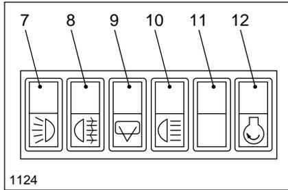
**7. Sidelight and Headlight** - Press bottom of switch to the first position to operate side, tail and panel lights. The lights in the other switches will illuminate. Press switch to the second position to operate the headlights. To switch lights off; press the top of the switch.
