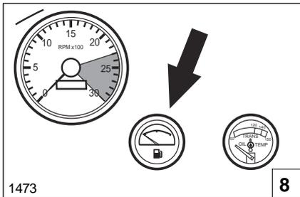
**8. Fuel Level** - Check fuel level gauge. Tank should be filled at end of each shift.
