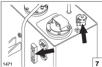
**7. Hydraulic Tank - Oil Level Check** - Operate the body hoist cylinders to their fully-extended positions to charge cylinders and lines then lower the body. With the engine off, the sight gauge should show half full. Add oil if low.
