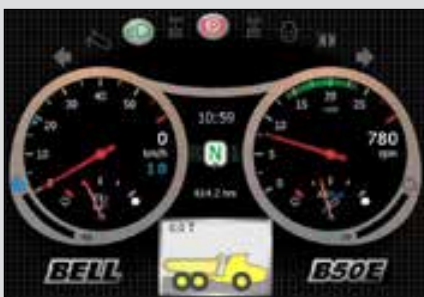
The exclusive on-board weighing presents the operator with real time information on the payload while the machine is being loaded. A 'speed restriction' mode can also be activated if the machine is significantly overloaded.
