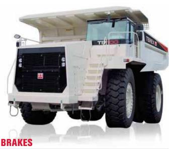
Service – All hydraulic brake system control. Transmission mounted pressure compensating piston pump provides hydraulic pressure for brakes and steering. Independent circuits front and rear. Each circuit incorporates a nitrogen/hydraulic accumulator which stores energy to provide instant braking response.
