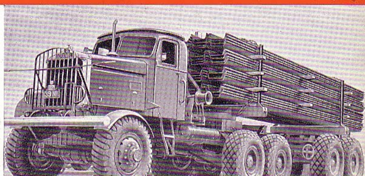
"Constructor" 15' 9" Wheelbase Oilfields Motive Unit with 80,000 lbs. line pull reversible winch and fifth wheel turntable for attaching semi-trailers.
