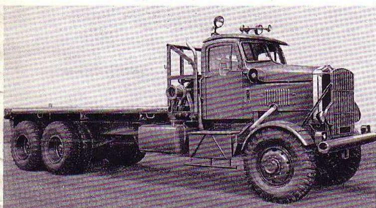
"Constructor" 21' 9" Wheelbase Oilfields Truck fitted with 50,000 lbs. line pull reversible winch, tail roller, headache rack and gin pole equipment. Load capacity 40,000 lbs.
