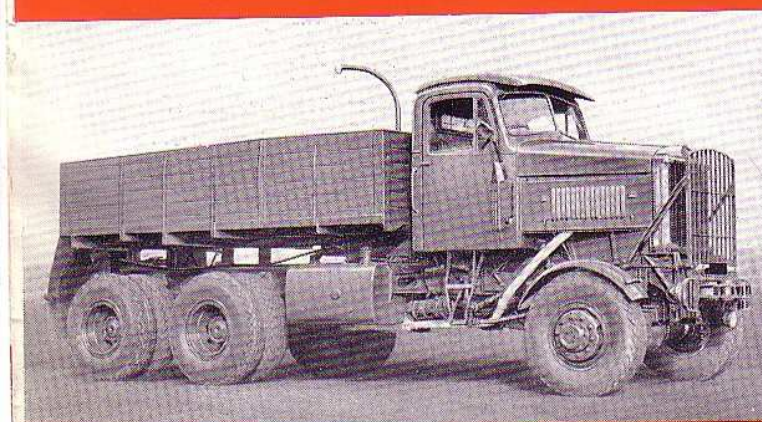
"Constructor" 15' 9" Wheelbase Heavy Duty Tractor with winch suitable for gross train weights of up to 336,000 lbs.
