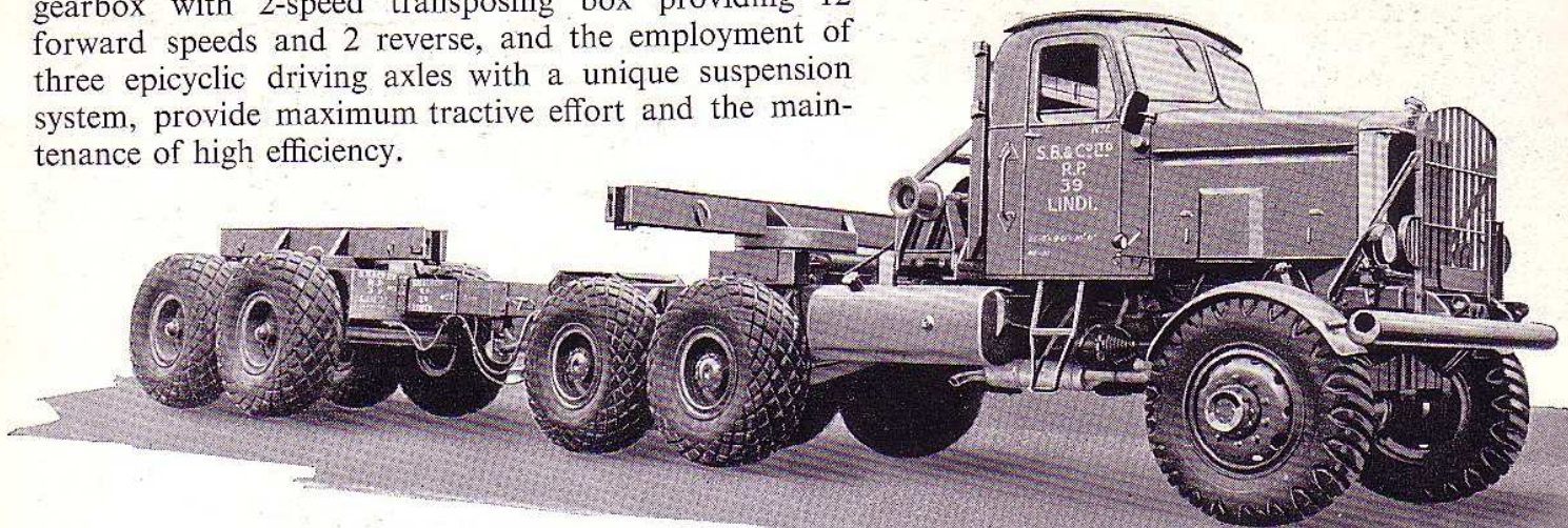
"Constructor" 15' 9" Wheelbase Motive Unit with extensible pole type semi-trailer for round timber haulage.
