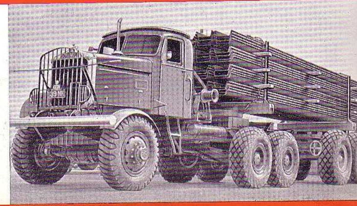
"Constructor" 15' 9" Wheelbase Motive Unit with extensible pole type semi-trailer for loads of abnormal length.
