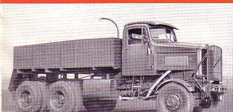
"Constructor" 21' 9" Wheelbase Oilfields Truck fitted with 50,000 lbs. line pull reversible winch, tail roller, headache rack and gin pole equipment. Load capacity 40,000 lbs.
