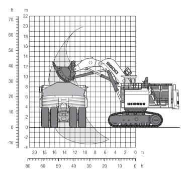
T 284 Mining Truck loaded by the Liebherr R 9800 hydraulic excavator in face shovel configuration
