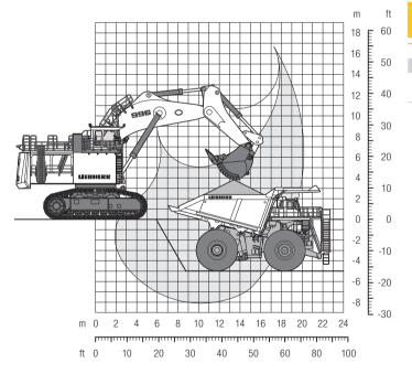
T 284 Mining Truck loaded by the Liebherr R 996 B hydraulic excavator in backhoe configuration
