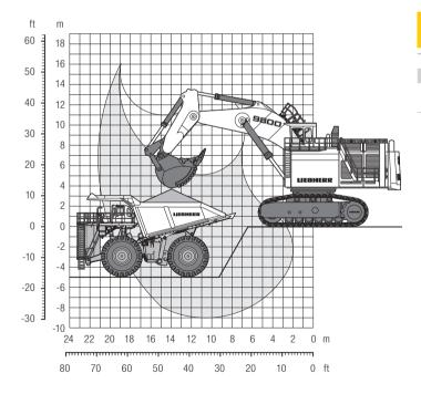
T 284 Mining Truck loaded by the Liebherr R 9800 hydraulic excavator in backhoe configuration
