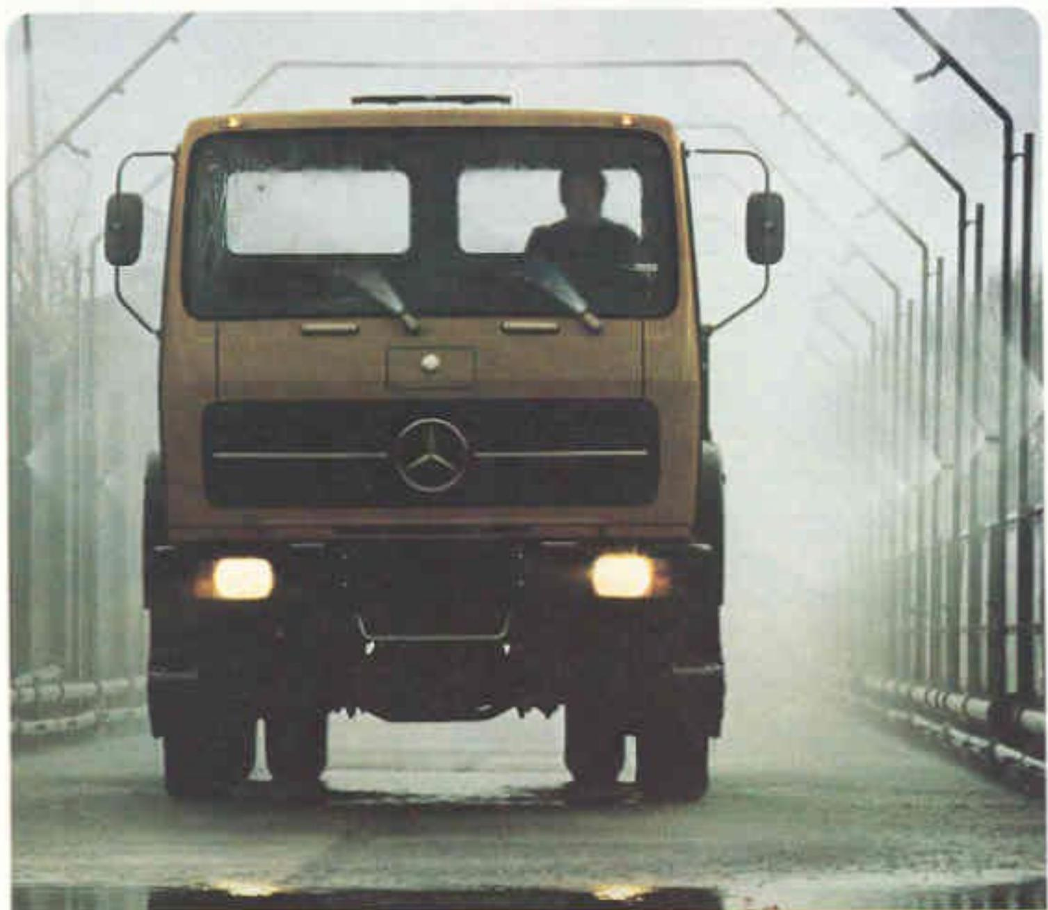
A 2-inch monsoon rain, about 70 litres of water per square metre, thrown onto the track at this test caused just to detect whether the floor, air intakes, doors or windows are leaking.
