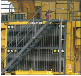
Komatsu's 960E-1 offers stairway access with entry from either the right or left side of the truck depending on the customer's preference.
